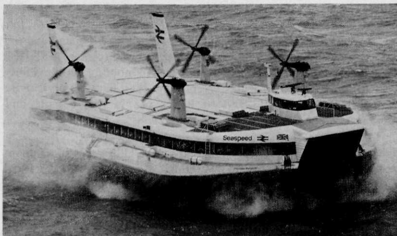
One of the SRN4s operated by Seespeed on the Dover Boulogne route in the Channel. With a top speed of 78 knots (148 km/h) these craft would have a high reinforcement capability in time of crisis; they can carry 254 passengers and 30 vehicles
