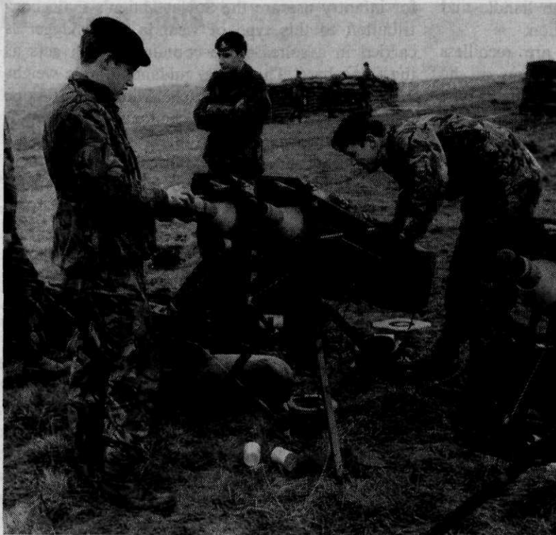
Vigilant being prepared for range firing; this man-portable wire-guided antitank missile system is lethal against the heaviest battle tank
