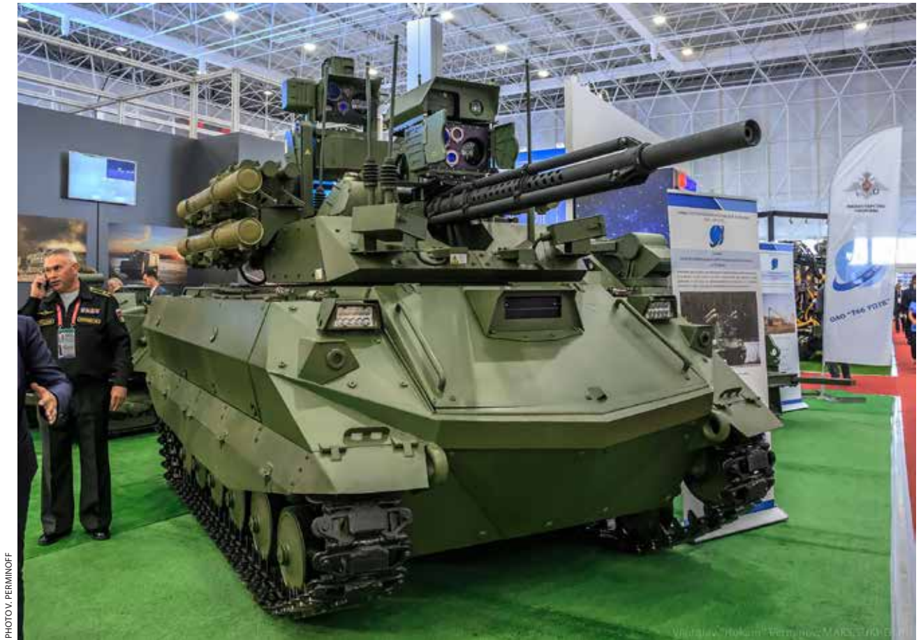
Russian URAN-9, a tracked unmanned combat ground vehicle
